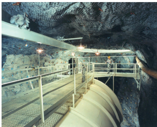
The underground tank where Brookhaven National Laboratory's solar neutrino experiment took place.
