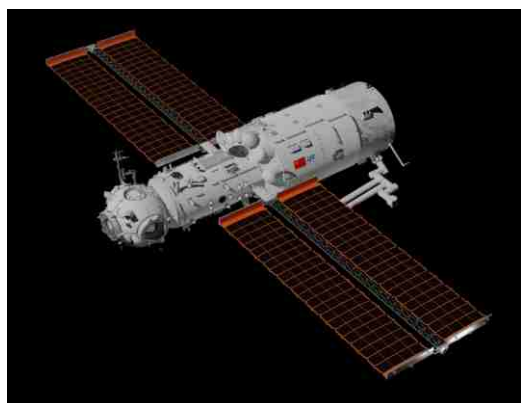
Tianhe core module with the robotic arm at the docking position (at the right end of the module)
