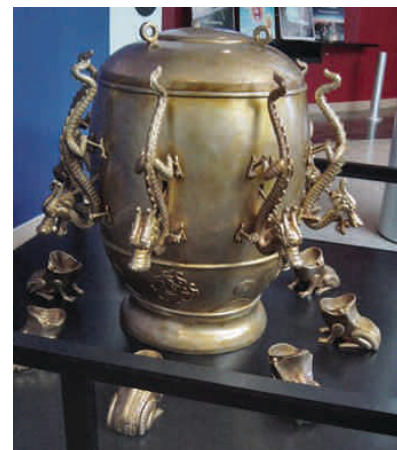
Replica of Zhang's seismoscope
