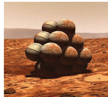
Mars Pathfinder landing with airbags
